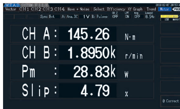
Motor analysis screen (Torque, rotation rate, motor power, slip) For CH B, enter the Z-phase pulse of the encoder to measure electric angle, and enter the B-phase pulse to measure rotation direction.
