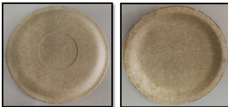
Fig. 8 – Biodegradable packaging from pineapple leaves with bio-coating solutions.
